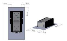
The unit can be wall mounted in a vertical orientation only with the connections at the bottom.
